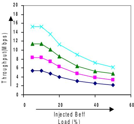
Fig. 5. Effect of injected Best Effort load on the throughput of ELINE traffic, no QoS
