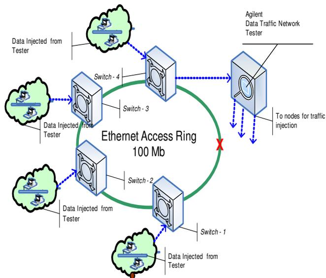
Fig. 3. QoS Test Bed.
