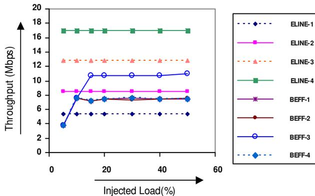
Fig. 8. Effect of total injected Best Effort Load on the throughput of ELINE traffic, with QoS applied.
