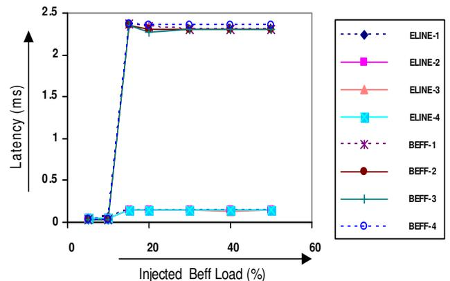
Fig. 7. Variation of latency with total injected load in the ring, with QoS applied.
