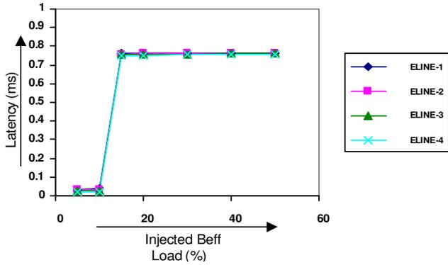
Fig. 4. Variation of Latency with total Injected Load in the ring, no QoS
