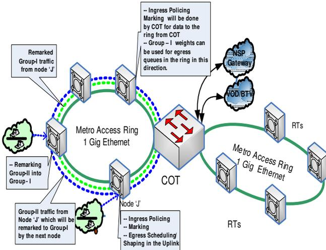
Fig. 1. Metro Ethernet Ring with Injected and Transit Traffic in different groups.
