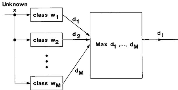
Fig. 1.  $d_1 = p(x|w_1)$ ,  $d_2 = p(x|w_2)$ ,  $\dots$ ,  $d_M = p(x|w_M)$ .  $d_i$  is the discriminant function for class  $w_i$ ,  $i = 1, 2, \dots, M$ .
