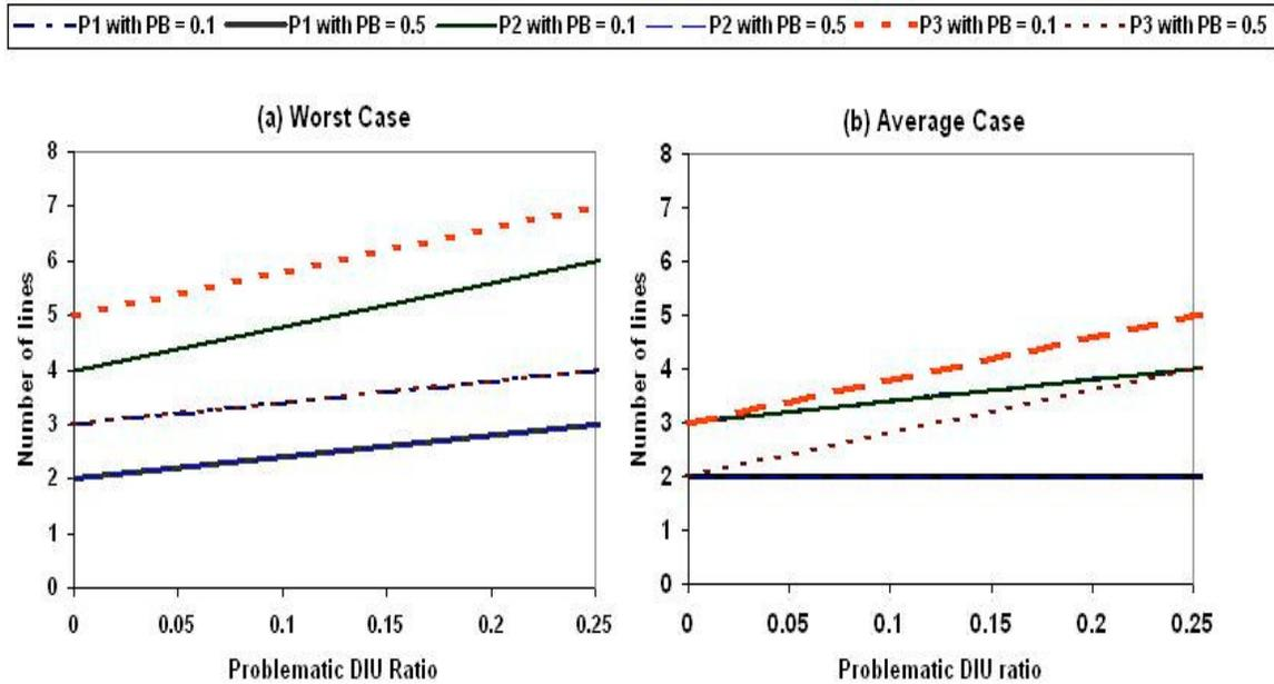
Figure 4-4 Number of telephone lines needed at NMS for different ratios of “Good and Problematic” NEs.
