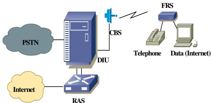
Figure 1-1 corDECT system architecture
