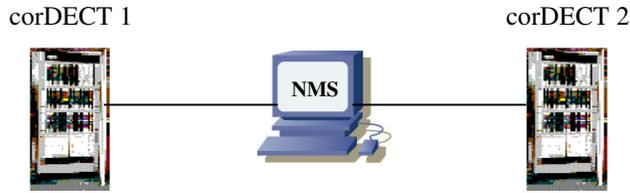
Figure 2-1 NMS and NE are connected through serial port
