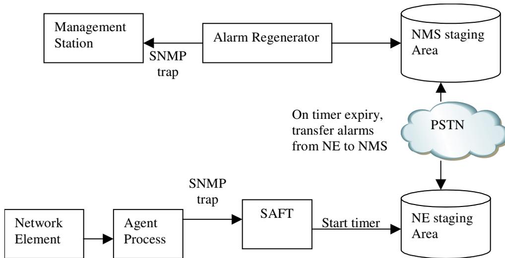
Figure 3-4 Alarm delivery mechanism
