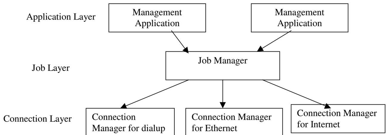
*Figure 5-1 Generic Software architecture for DCN*
