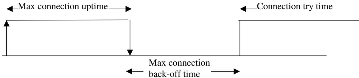
Figure 3-3 Timers used in connection maintenance
