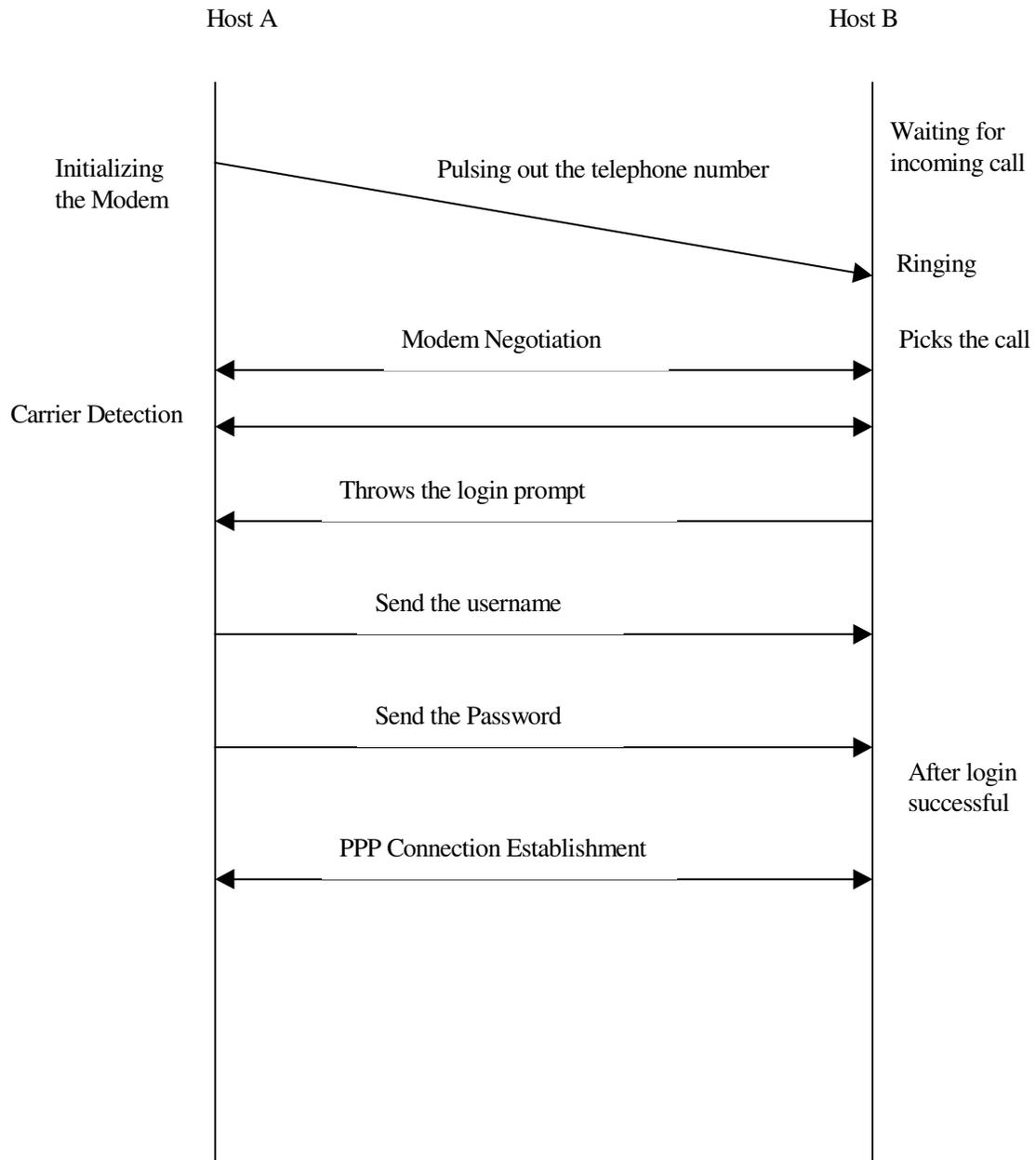
Figure 2-6 Stages in establishment of a Dialup Connection
