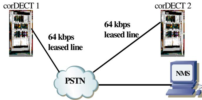
*Figure 2-3 NMS and NE are connected through private leased lines (ISDN, X.25)*
