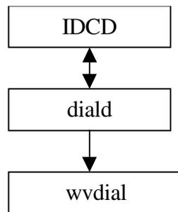
Figure 5-6 Block Diagram of dialup connection manager
