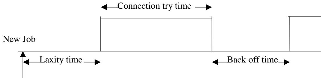
Figure 3-2 Timers used in connection establishment
