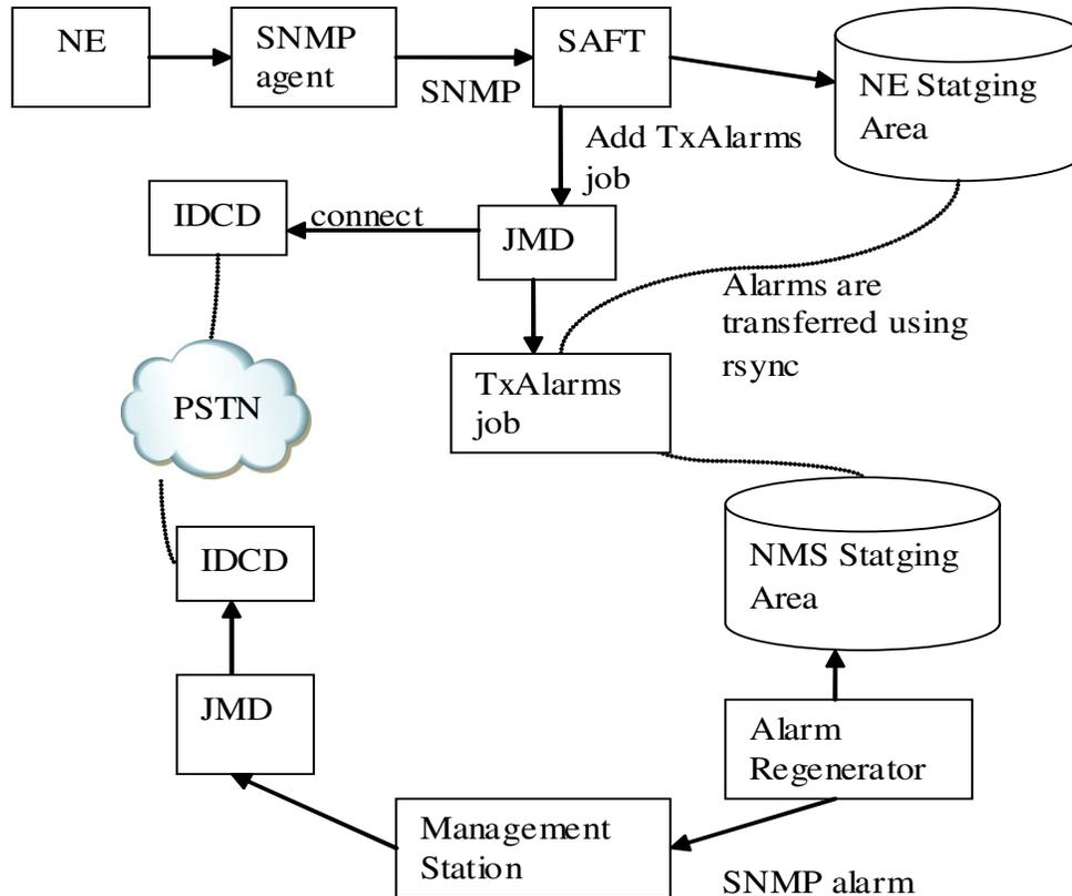
Figure 5-9 Block diagram for delivering the alarms to NMS
