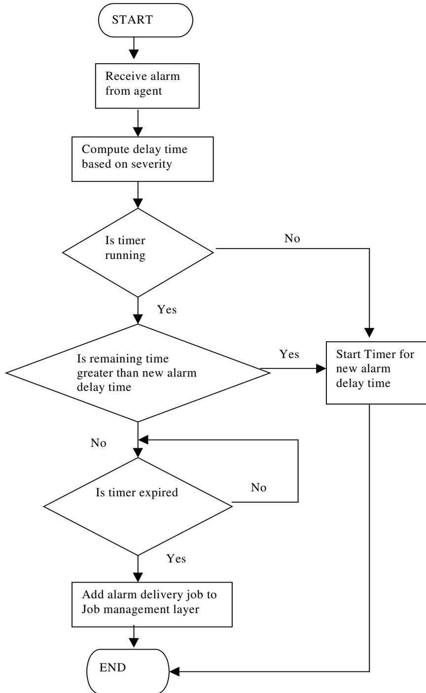
Figure 5-10 Flow chart for alarm delivery mechanism
