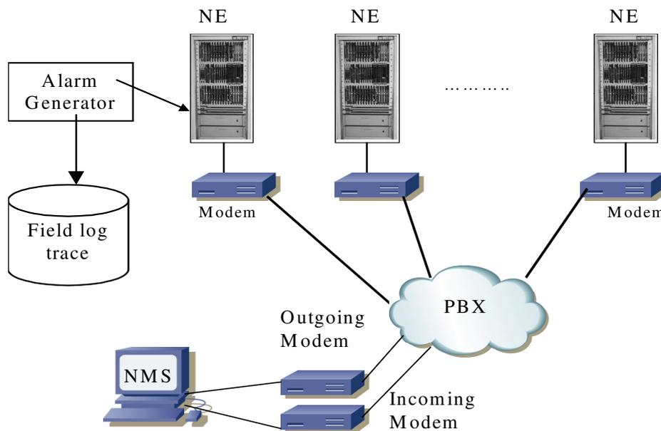
*Figure 4-2 Lab experiment setup for measuring the blocking probability*
