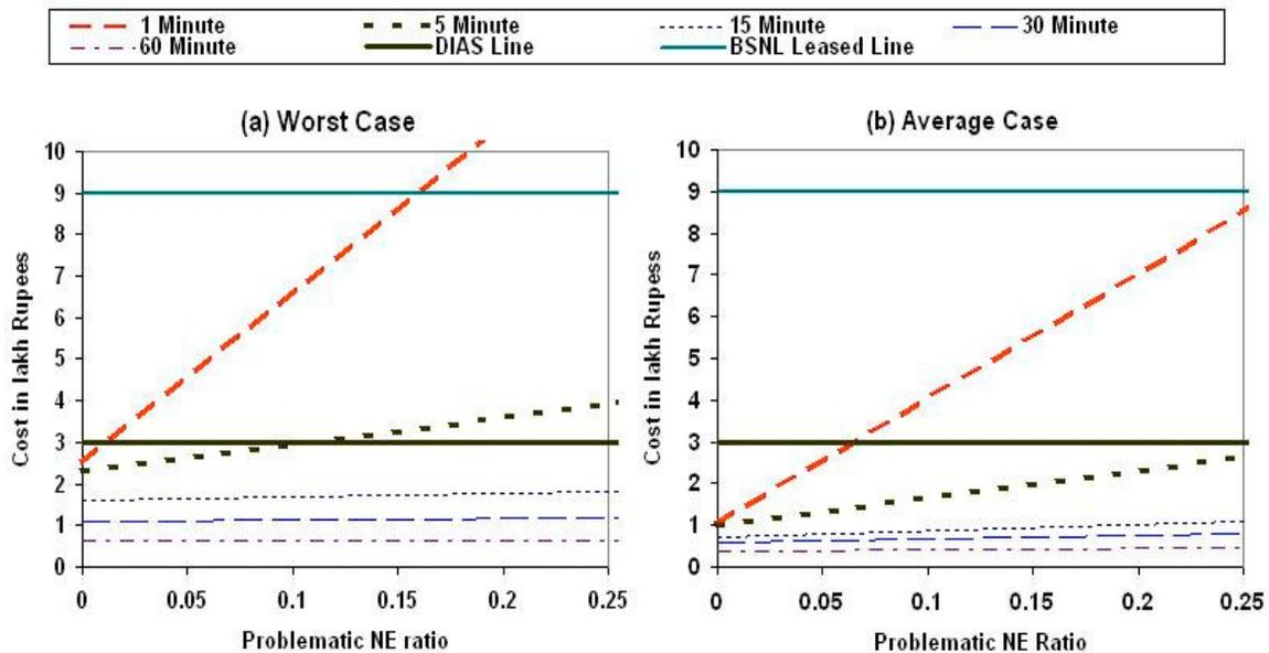
Figure 4-6 The dialup monthly cost in lakh of Rupees for different ratios of problematic NEs. Figure shows the worst case and average case scenarios. Different series are drawn for different desired response times for critical alarms
