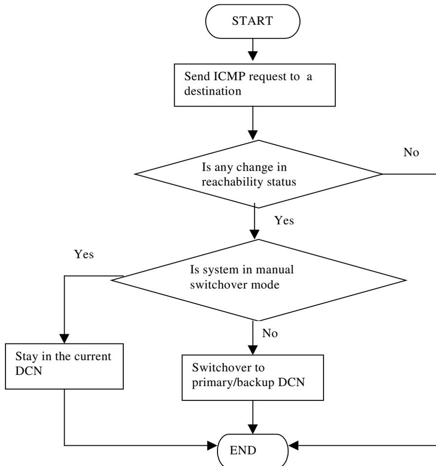
Figure 5-4 Flow chart for DCN backup mechanism
