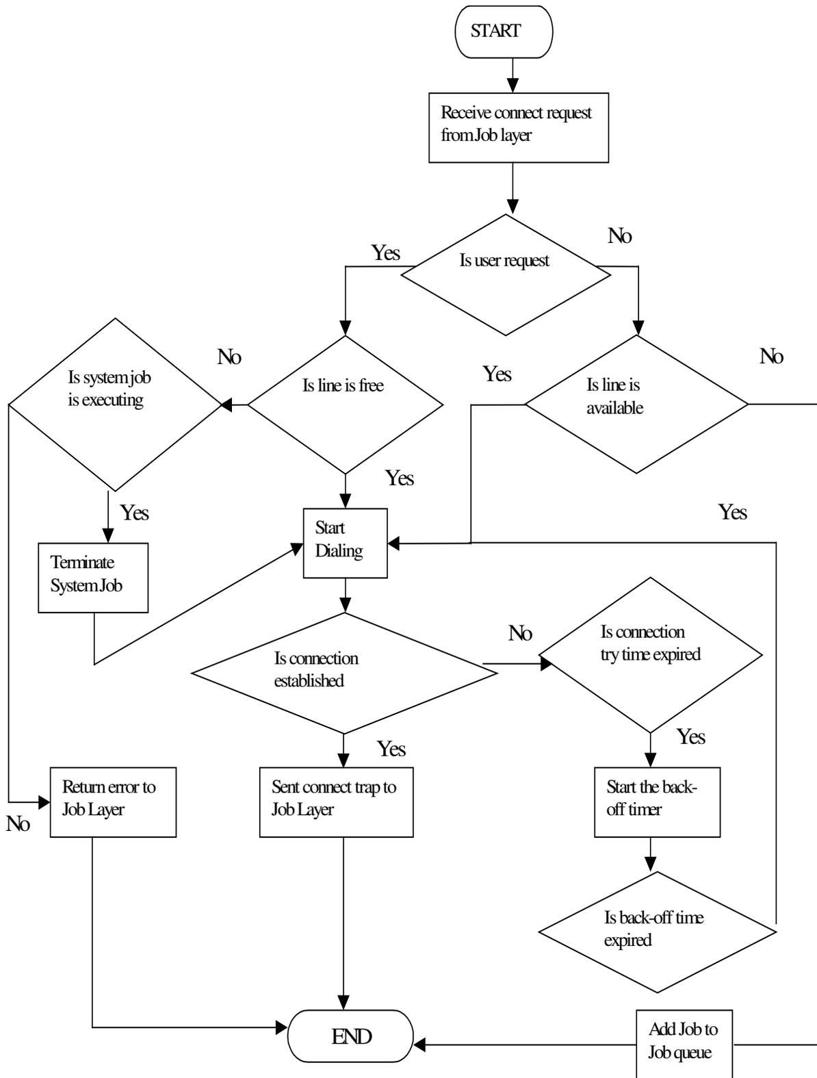
Figure 5-7 Flow chart for the dialup connection establishment
