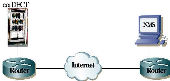
*Figure 2-4 NMS and NE are connected through Permanent IP*
